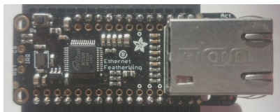
Figur. 3. Ethernet-kort, Ethernet FeatherWing [3]
