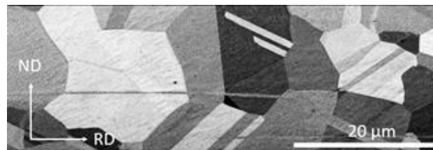
Figure 4.21: SEM image of rectangular ND-RD specimen using a BSE detector at 2400x magnification.
