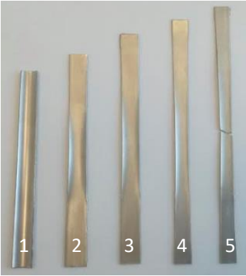
Figure 4.13: Image of the five tubular specimens ordered from zero strain to fracture.
