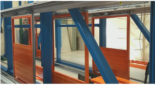
Figur 1: The door used for testing at ASSA Abloy, model SL500 with adjustable weight.
