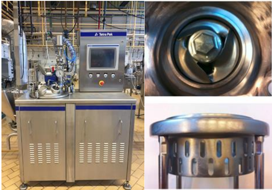
Figure 4: Tetra Pak High Shear Batch Mixer (25 litres), on the left side of the mixer is the vessel and on the right side is the display unit. b) (top view) rotor and stator, c) Stator with slots 5x14mm
