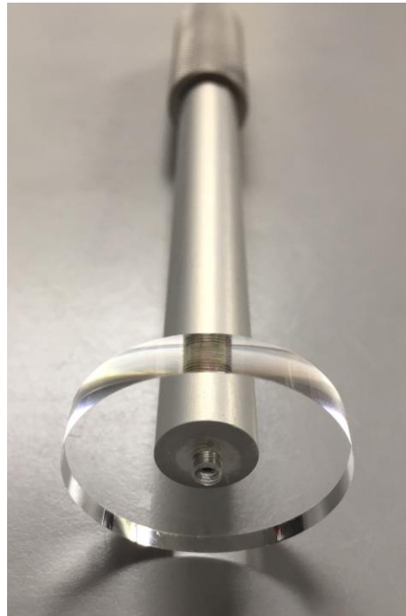
Figure 4: a) Texture Analyser (TA-XT2i, Stable Microsystems, UK, Godalming). b) Disc Plunger Probe used for the texture analysis.
