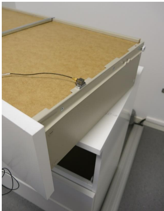
Figure 3.29 Vibration detector mounted at the pre-drilled front hole of the DL slide.
