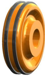
Figure 5.32. POM material marked in orange and two soft strings of TPE-E marked in black.
