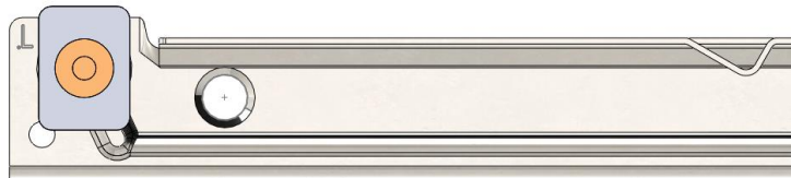
Figure 5.13. Modified drawer slides with blocks instead of wheels.
