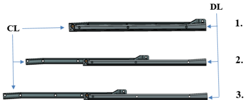
Figure 3.14 Description of the opening and closing mechanism of the roller slide.
