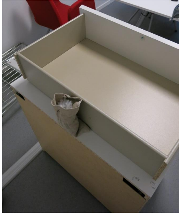
Figure 3.27 The damper placed at the back of the drawer that will be used for the test.
