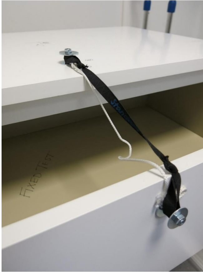
Figure 3.24 Bolts, nuts and washers keeping the two bands in place.
