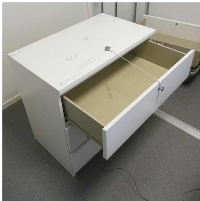
Figure 3.23 Start position of the test determined by the inelastic white band.
