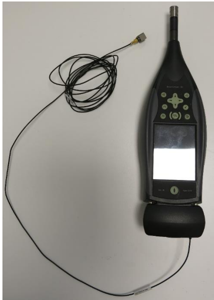
Figure 3.28 Vibration detector connected to the decibel meter.
