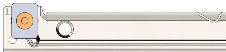
Figure 5.17. Modified drawer slides with blocks instead of wheels.
