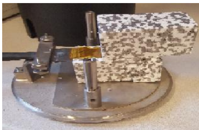
Figure 18 Typical set-up for TPS measurement
