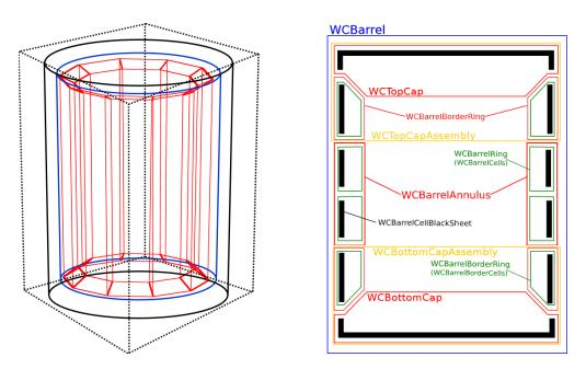
Figure 7: 3D and 2D diagrams of a simulated water Cherenkov detector via WCSim, taken from Ref. [18].
