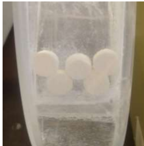
Figure 2.9: . Tablets in the drum after the end of the friability test.
