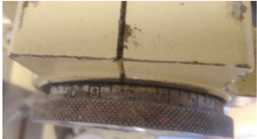
Figure 2.5: The rotor adjusts the pressure of the press.
