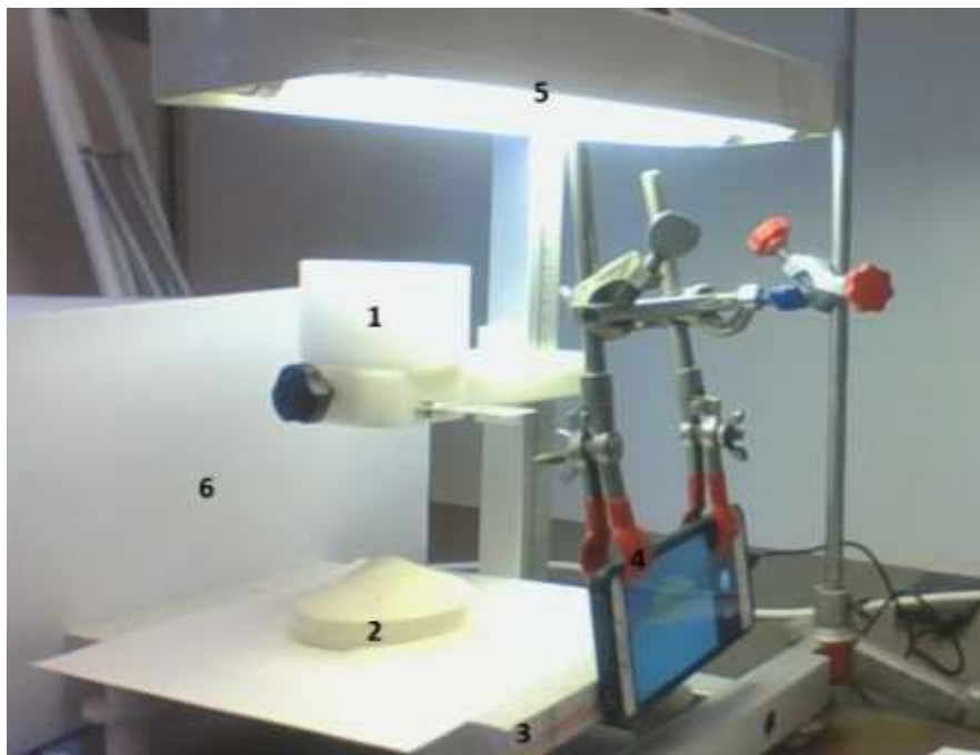
Figure 2.1: The set-up that was used to measure the angle of repose. 1) funnel 2) petri dish 3) marble bench 4) stand with fixed camera 5) light 6) white background.
