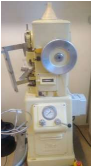
Figure 2.4: Tableting press at the Department of Food Technology.
