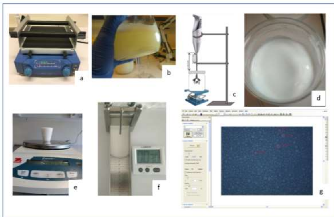
Figure 2.11: Procedures and equipment used in dispersion and foam preparation and characterization. a) orbital shaker, b) dispersion, c) set up of the blender, d) foam, e) weighing the foam in a plastic cup of 46 dL f) consistometer g) bubble diameter measurement using optical microscopy.
