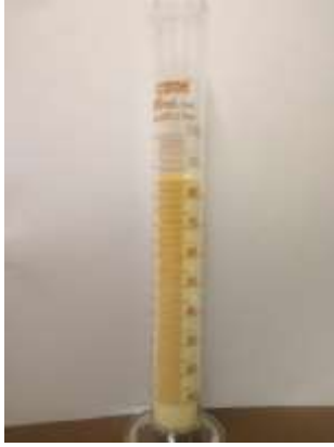
Figure 2.3 A volumetric cylinder with powder after tapping (initial volume or free flowing volume was 100 ml).
