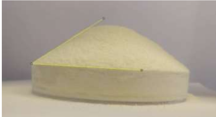
Figure 2.2: An example of a picture taken by the set-up of figure 2.1. The angle of repose was measured by using the software ImageJ .
