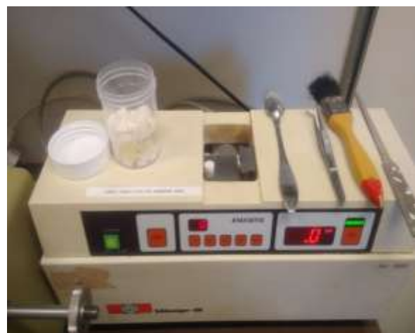
Figure 2.7: Tablet hardness tester. For measuring hardness over 5 kPonds.
