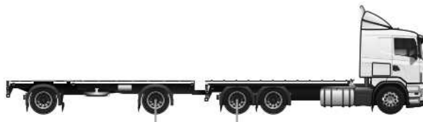
Figure 3.5: A tractor unit where swap containers can be placed (Transportstyrelsen, n.d.)
