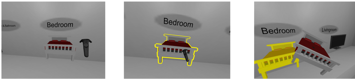
Figure 4.10: The different highlighters used for product interaction. Left picture: no interaction with product. Middle picture: hand controller touching a product. Right picture: user grabbing and moving the product. The yellow highlighter showing the initial position for that product.
