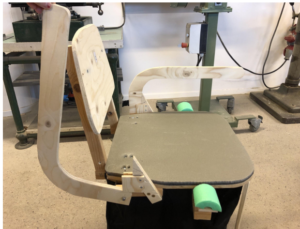
Figure 3.17 Early prototype of chair and function for rotating the seat by pressing levers (green) downwards.
