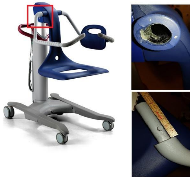
Figure 3.11 The figure to the left show Alenti. The upper right image show the point of attachment for the armrest in detail. Its position on Alenti is marked with a red box. The lower right image shows the armrest when removed from the chair, and what the locking mechanism looks like. Image of Alenti (Arjos, 2019)
