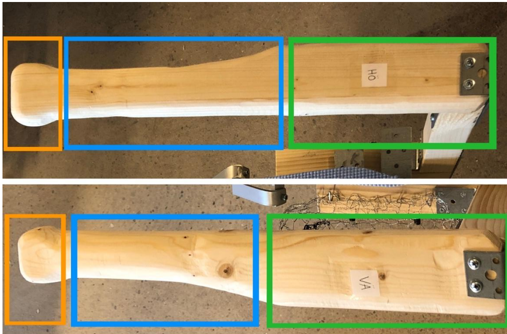
Figure 3.9 The two armrests used in the final user test, with the right armrest at the top and left at the bottom. The width and length are seen from an above view and the thickness is going into the paper. The front of the armrest is marked as orange and 60 mm wide. The narrower gripping part is marked with blue, 50 mm wide, and the wider supporting area is marked with green colour, 70 mm wide.
