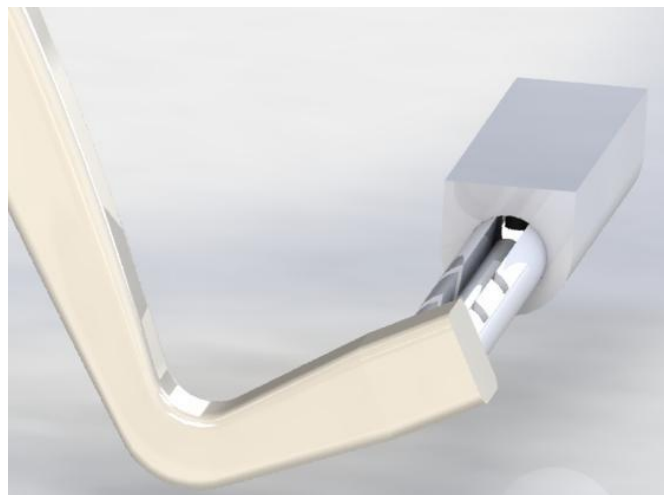
Figure 3.12 The image shows how the armrest is fastened to the chair. There are two slots on the armrest to be able to adjust the width between them.
