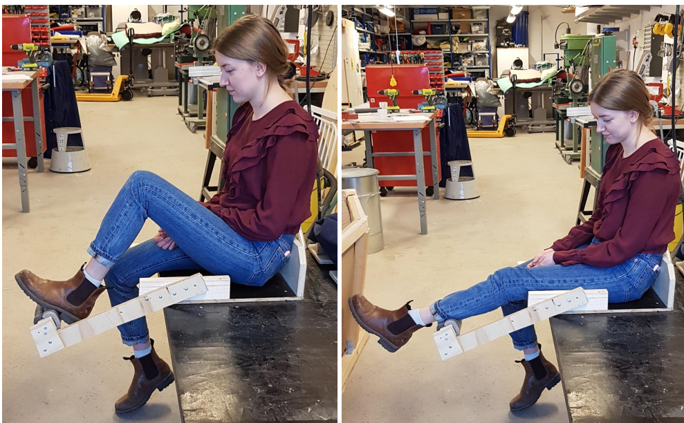
Figure 3.29 The pictures show how the foot support can be used, with either the foot on or the calf.
