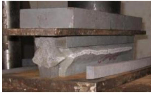
Figure 40: Plastic brick compressed and deformed (Sierra Jiménez 2016)
