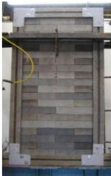
Figure 35: Full-scale plastic wall tested for lateral static load (Sierra Jiménez 2016)
