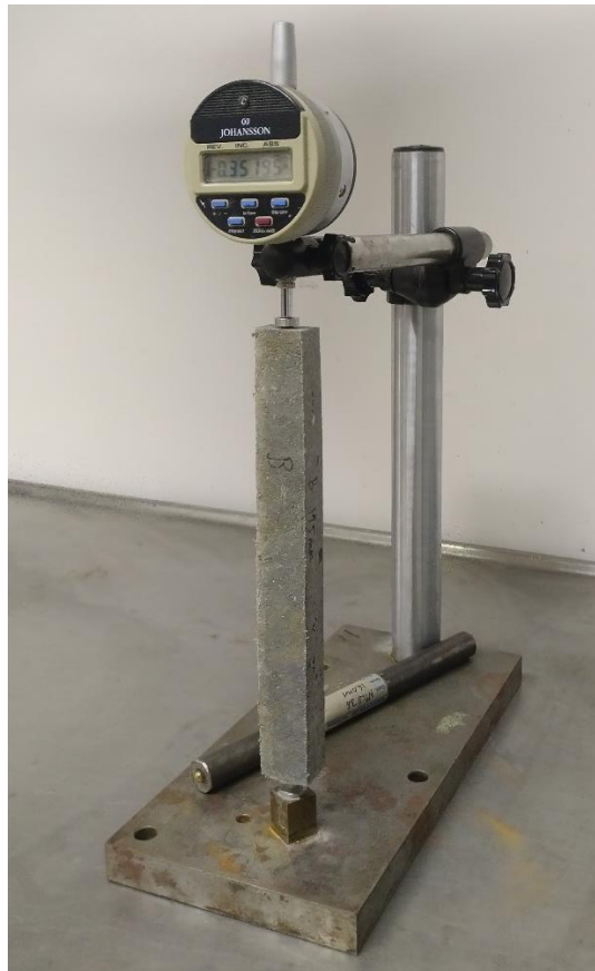
Figure 28: Test of the thermal expansion coefficient (Photo: Lars Wadsö, 2019)
