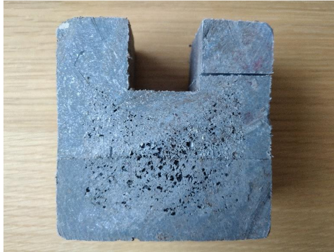
Figure 37: Plastic sample extracted for measurement of heat capacity and thermal conductivity (Photo: Lars Wadsö, 2019)
