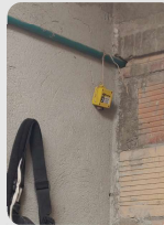
Figure 7. Installing Tiny Tag in masonry house.
