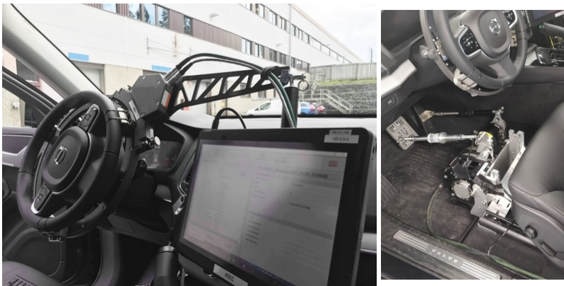
Figure 4.2 (Left) The steering robot used in the experiments. (Right) The pedal robot used in the experiments.
