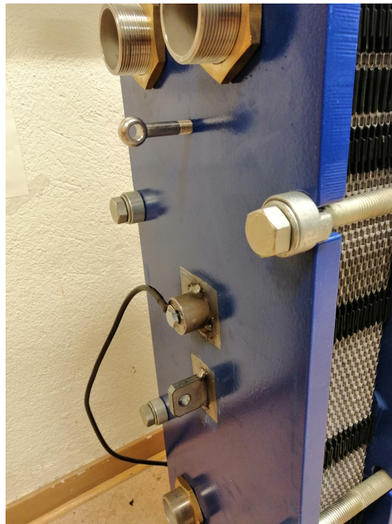
Figure 32: The three designs related to the frame plate. The black cable connected to the FP boss is the "simulated" ground cable which in reality is connected to a ground embedded rod.
