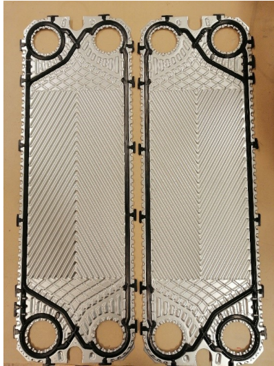
Figure 20: Corrugated plates with gaskets. Two adjacent plates are shown, illustrating how the gasket layout alternates between two patterns to make sure that the two fluids never mix
