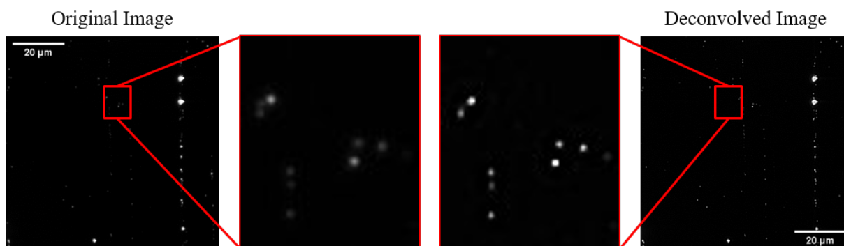
Figure 5.2: PSF estimation with images of 100 nm sized beads ( \rightarrow small dots).
