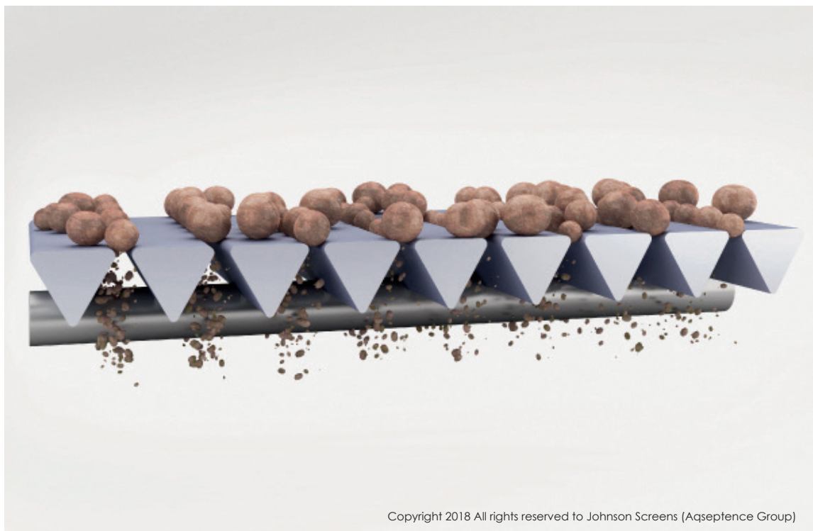
Figure 3.8. Principal sketch of Johnson Screens patented vee-wire® screen technology that is implemented in the Triton Underdrain™ design (Figure published with kind permission from Aqseptence Group 2017).
