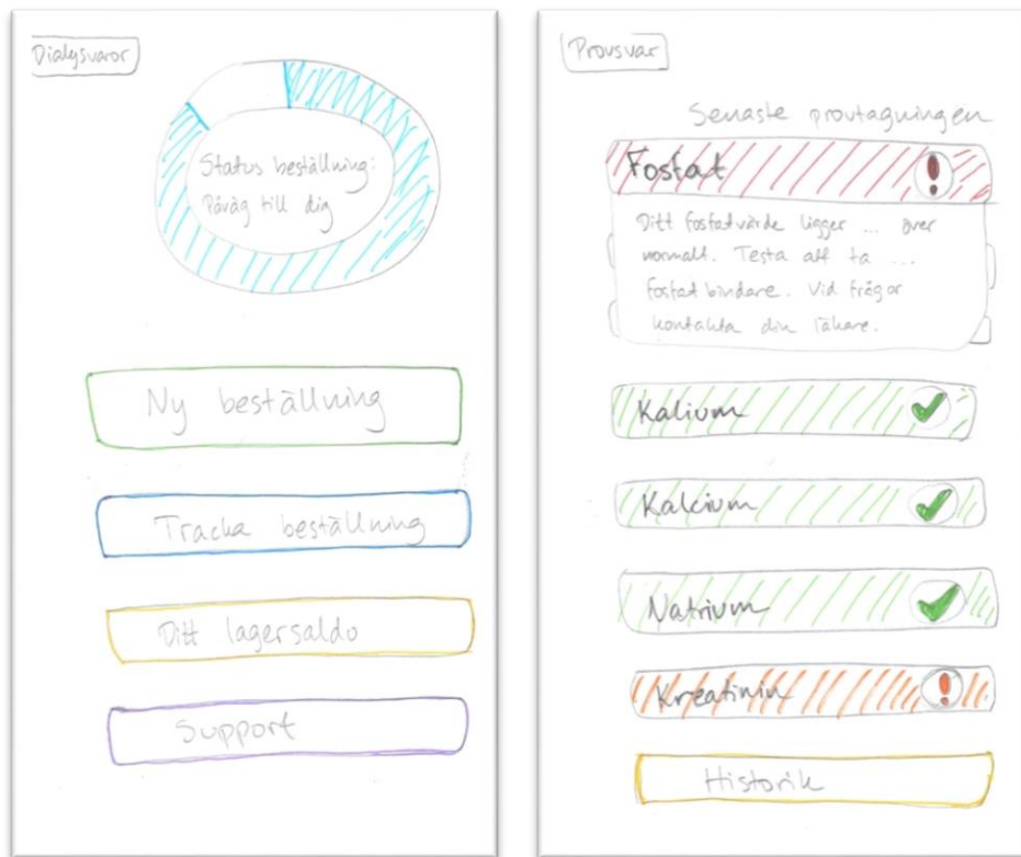
Figure 11. Two of the sketches from concept one. The left-hand sketch shows functionalities related to ordering. The functionalities are divided into four different buttons, four different paths. The patient can either make a new order (Ny beställning), track an order (Tracka beställning), check the home stock (Ditt lagersaldo), or get support (Support). The right-hand sketch presents the patient's last blood test results and related information.
