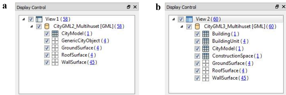
Figure 22. Feature types of the CityGML2.0 (a) and 3.0 (b) in the Multihuset Bryggan model
