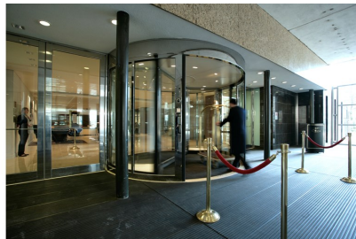
(b) The Revolving door has rotating pockets that let people through.
