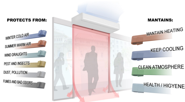
Figure 2.10: The air curtain and its advantages when placed above an entrance are shown [airtécnicos, n.d.] .
