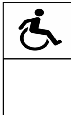
Figure 3.1: The activation button described in Scenario A. Depending on which part you press the hold open time will be long or short.
