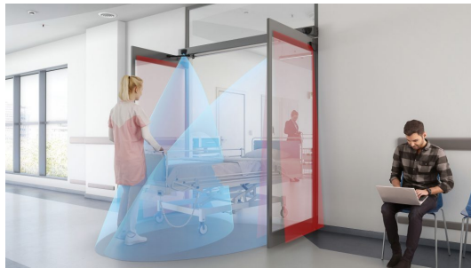
Figure 3.6: Two sensors are scanning the whole doorway. One sensor creates the safety zone, the red area near the door leaf. The other sensor is used to optimize the opening by over viewing the doorway, blue area [BEA, n.d.] .
