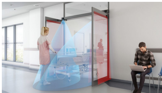
Figure A.8: Two sensors are scanning the whole doorway. One sensor creates the safety zone, the red area near the door leaf. The other sensor is used to optimize the opening by over viewing the doorway, blue area [BEA, n.d.] .
