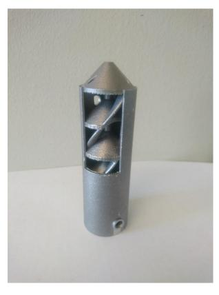
The technology of 3D printing has huge potential of creating a smarter and better heat exchanger. If the heat exchanger can be made smaller but with the same output this could have big impacts on cost and more importantly it is more sustainable. Less energy needed to have the same effects means less emissions. It could be used in everything from industry and refineries to home applications such as home brewers wanting a better way to cool their latest batch of beer.
