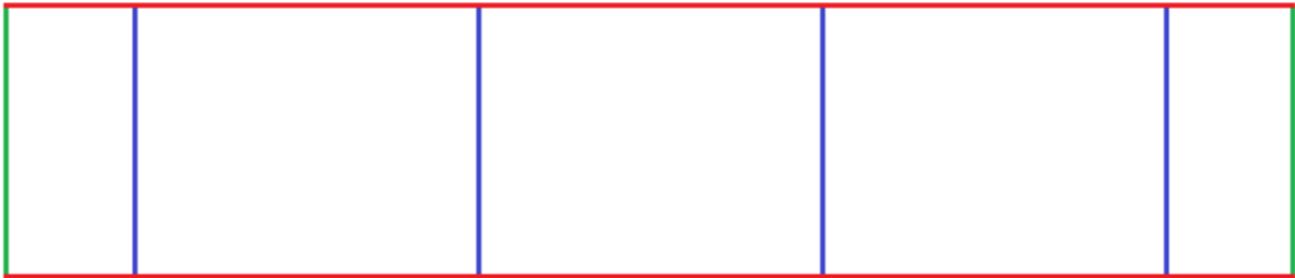
Figure 5.2: Layup locations seen at the cross-section of the bridge: Red: Top and bottom, Blue: Web, Green: Sides.
