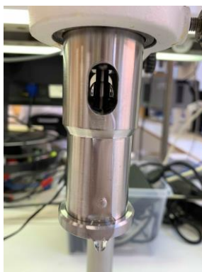
Figure 57 Cup containing the liquid sample for viscosity analysis.
