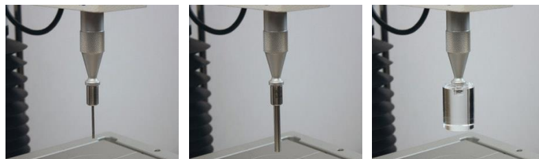
Figure 15 Probes used in mechanical tests – puncture probes (2 mm, left) and (5 mm, center), compression probe (36 mm cylinder).
