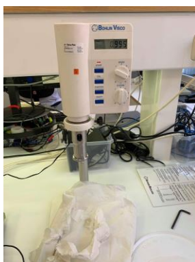
Figure 58 Measurement of viscosity using Bohlin viscometer.
