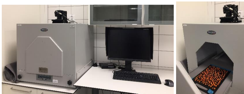
Figure 22 Digi Eye – the apparatus used in capturing images of the particles.
