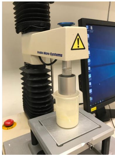
Figure 3.6 Picture of texture profile set up with cylinder probe
