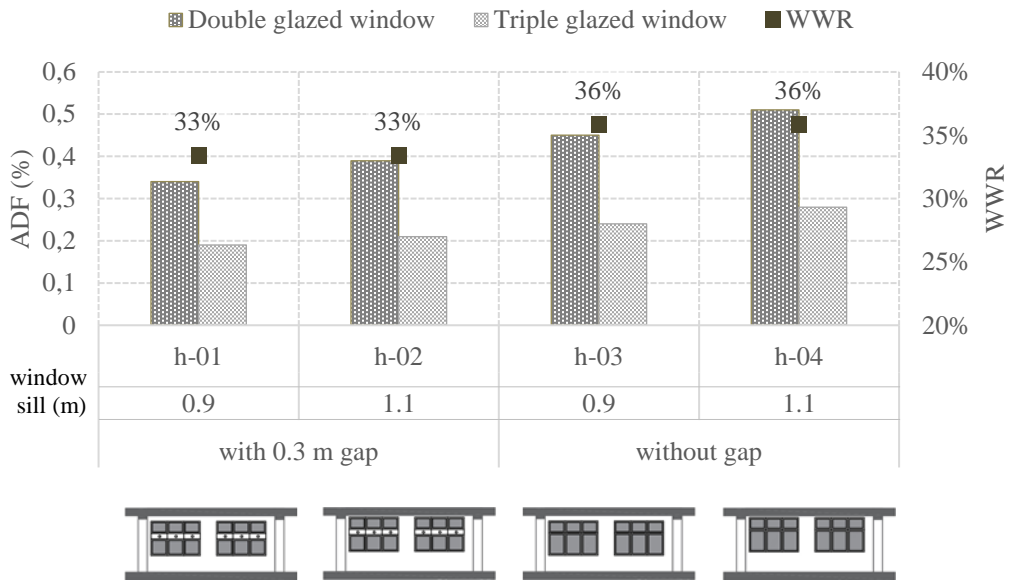
Figure 24: ADF (%) for horizontal shape variations with individual clerestory on the first floor.
