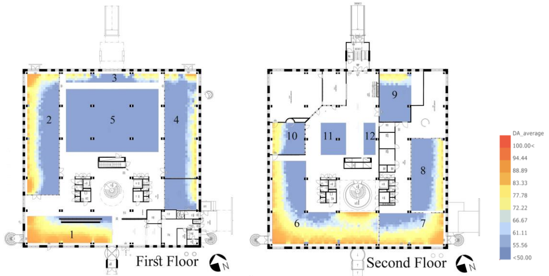
Figure 41: CDA_{300} by combination - BC of internal zones: 1. Cafeteria; 2. Biblioteket; 3. Computer space; 4. Silent study area; 5. Mid study area; 6. L-shaped study area; 7. Staff office-1; 8. Staff office-2; 9. Book store; 10. Conference; 11. Small study-1; 12. Small study-2.
