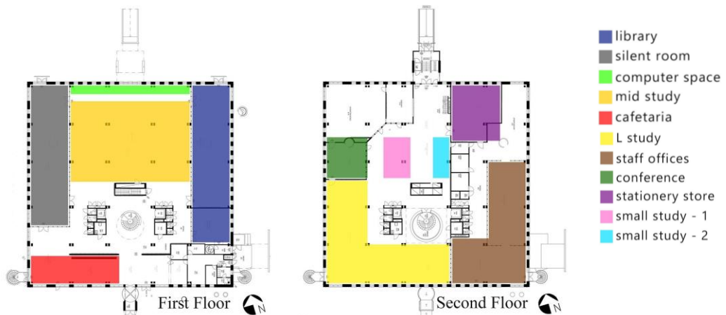
Figure 21: Daylight zones on each floor.
