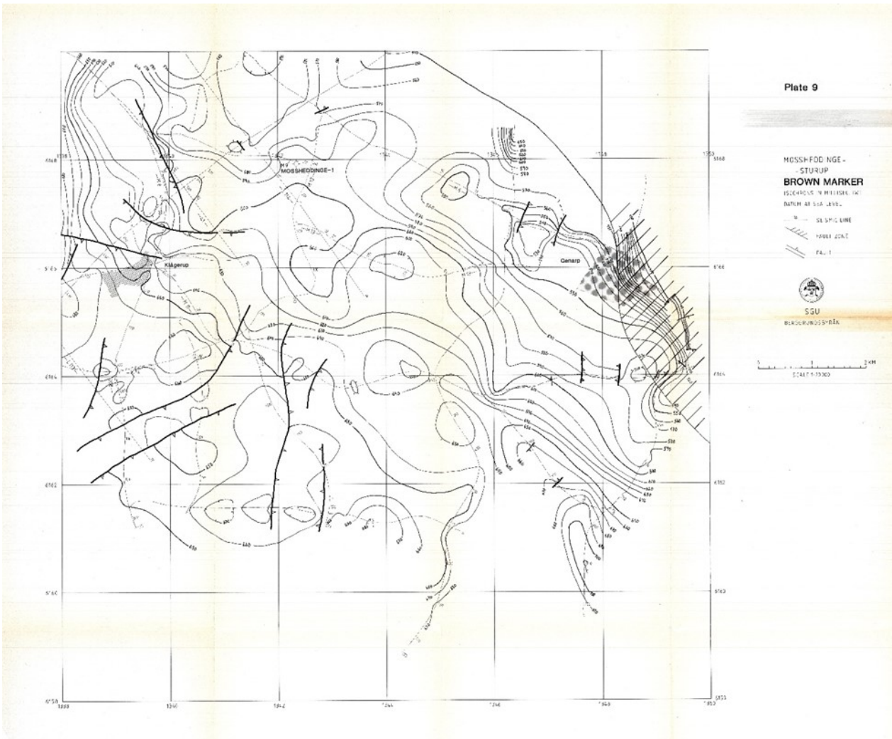
Appendix 6. Isochron map showing the depth of the Brown Marker in the Mosssheddinge-Sturup area (Larsson & Kumpas 1982).
