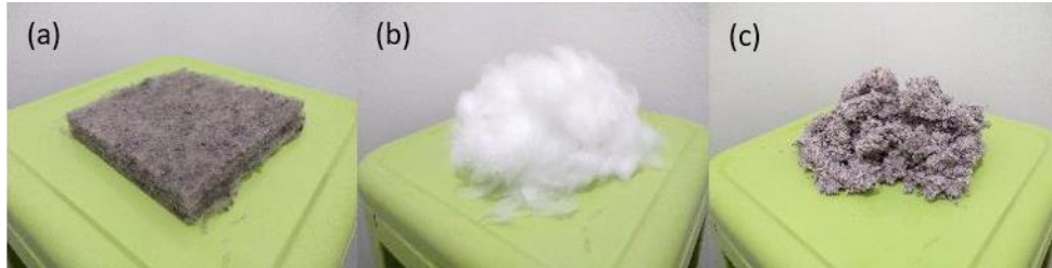
Figure 9. Insulation materials: (a) PET, (b) PLA, (c) CIF
