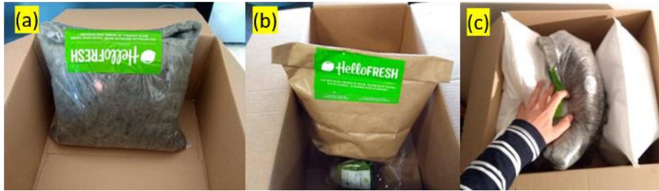
Figure 19. CPs in HelloFresh Box (a) PET CP, (b), Paper CP and (c) PLA CP.
