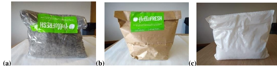
Figure 1. (a) PET CP currently used by HelloFresh, (b) Paper CP, (c) PLA CP.
