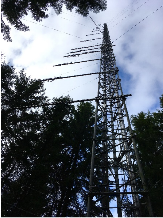
Figure 5. Instruments on the tall tower in Hyltemossa. Net radiation is measured on a boom pointing in a different direction than the other instruments. Photo by Iris Mužić.
