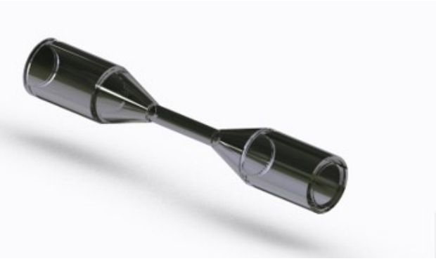
(b) Visualization of the 16 mm pipe from CAD drawing using PTC Creo.
