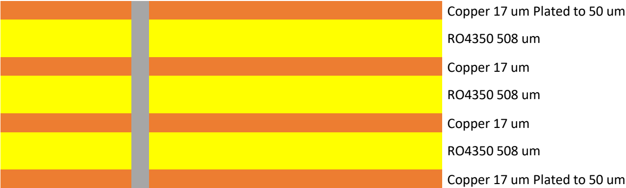
Via diameter 0.6 mm top to bottom
