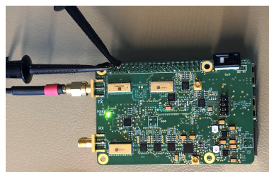
Figure 7.2: TX Output Test Setup.
