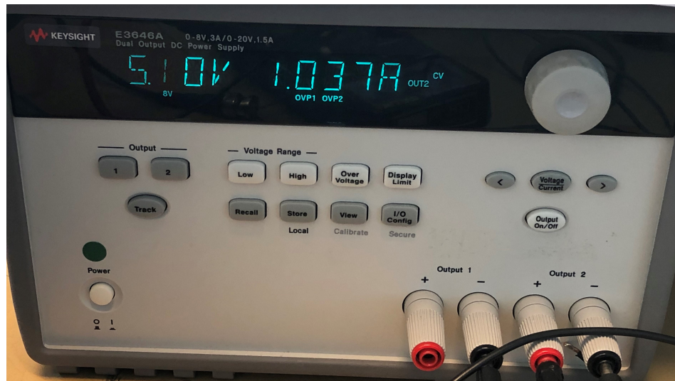
Figure 7.1: DC Supply Full Load Testing.
