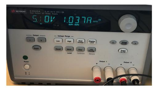
Figure 7.1: DC Supply Full Load Testing.
