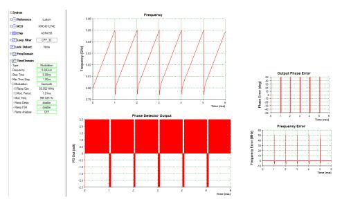
Figure 5.3: Simulation of ADF4158 PLL and HMC431LP4 VCO Synthesizer.
