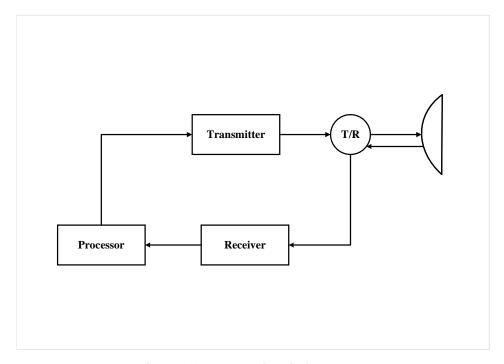
Figure 2.1: Basic Radar Block Diagram.
