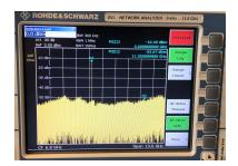
Figure 7.5: Spectral Measurements of TX Output Port After Modifications.
