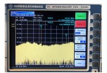
Figure 7.3: Spectral Measurements of TX Output Port.
