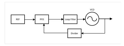
Figure 5.2: Basic Block Diagram of PLL Synthesizer.
