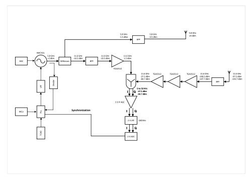
Figure 3.8: Radar System Block Diagram Version 3.
