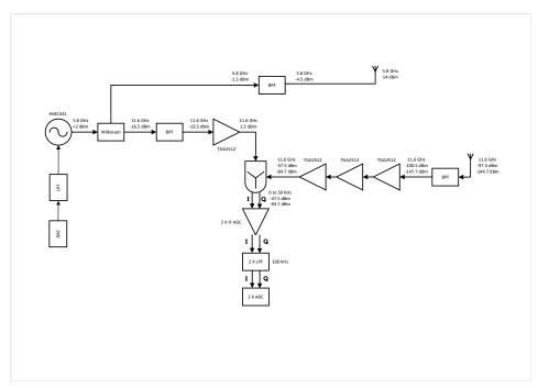
Figure 3.7: Radar System Block Diagram Version 2.
