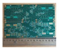
Figure 6.2: Harmonic Radar PCB Boards.
