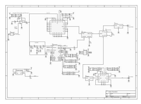
Figure 5.1: Radar Transmitter Schematic Diagram.
