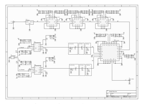
Figure 5.4: Radar Receiver Schematic Diagram.
