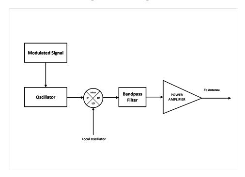
Figure 2.2: Radar Transmitter Block Diagram.
