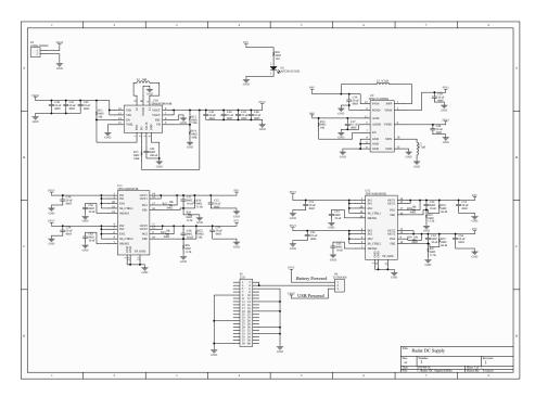
Figure 5.6: Radar DC Power Supply Schematic Diagram.
