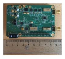
Figure 6.5: Harmonic Radar After Assembly.
