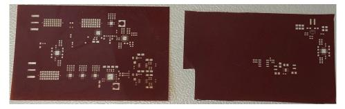
Figure 6.3: Top and Bottom Layers Stencils Using Flexible Film.
