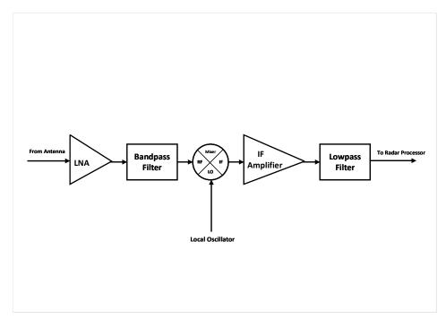
Figure 2.3: Radar Receiver Block Diagram.
