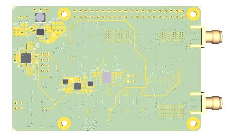
Figure B.2: RF Bottom Layer Layout.
