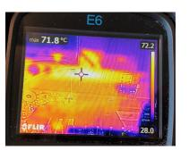
Figure 7.13: Thermal Image of the RX LNAs After Modifications.
