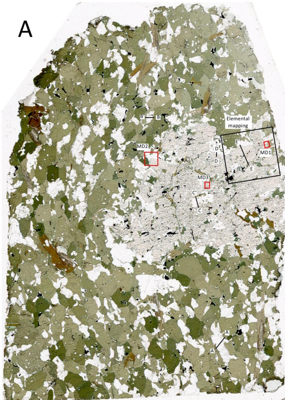
Fig. 4. Scanned photographs of the three thin sections; A, B and C. All three thin sections were examined using a polarization microscope and SEM-EDS analysis was made of thin section A. The three micro domains chosen for P-T calculations (MD1, MD2, MD3) are marked with red squares, the profiles of plagioclase and garnet are marked with black lines and the location for elemental mapping of the garnet rim (Appendix 2a), for the purpose of investigating possible zonation, is marked by a black square.
