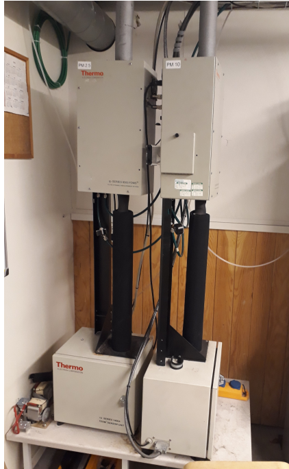
Figure 25: Field test reference instrument TEOM 1400AB with 8500 FDMS located in Dalaplan, Malmö. Unit on the left measures PM 2.5 and unit on the right PM 10.
