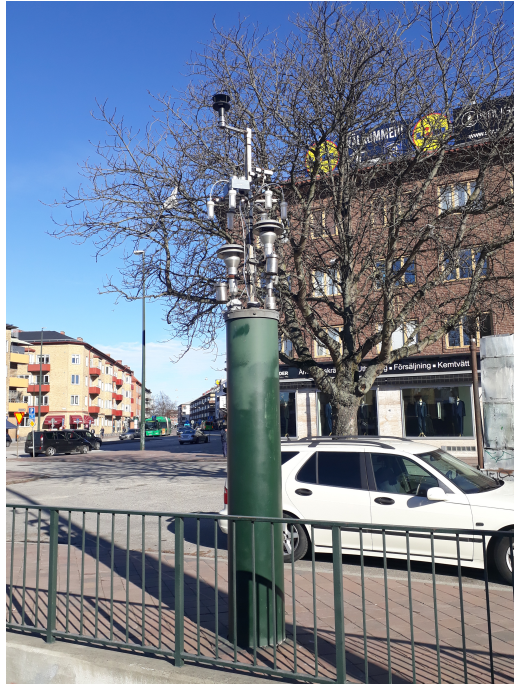
Figure 24: Inlets of the air measurement station in Dalaplan. Mushroom shaped inlets are the cyclonic separators for PM sampling.
