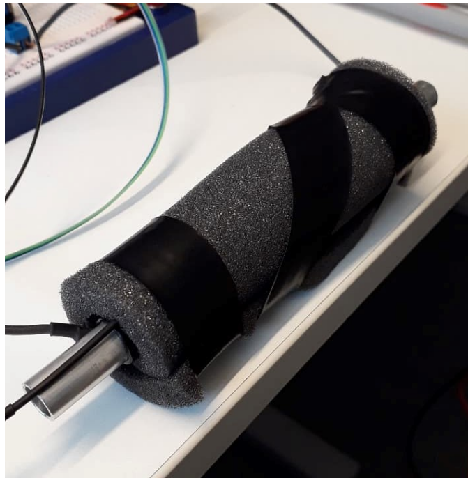
Figure 16: Heating pipe isolated with 1 cm thick polyurethane foam.
