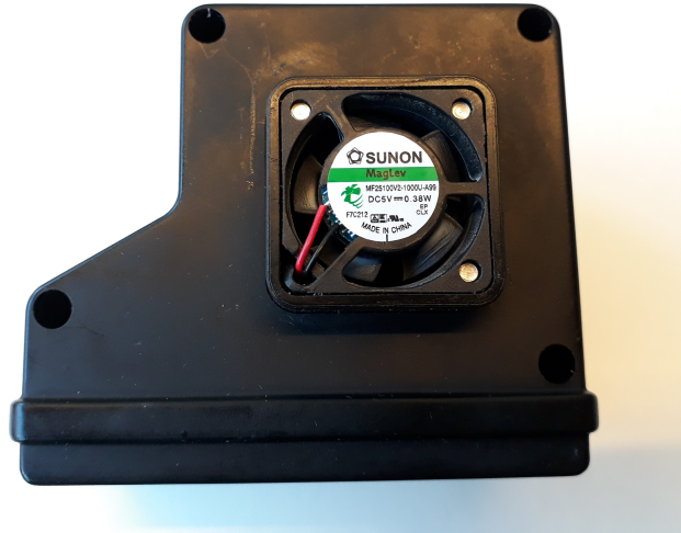
Figure 5: Small fan on the OPC-N2 that creates the airflow through the sensor.
