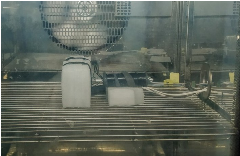
Figure 18: Initial prototype during the climate tests. Sensor wrapped in white isolation(on the left) with the heating pipe(on the right) which supported by a white block to keep the airflow line horizontal.
