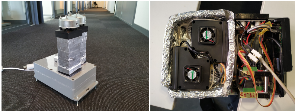
(a) Outside, the two towers are heaters with inlet at the top.
