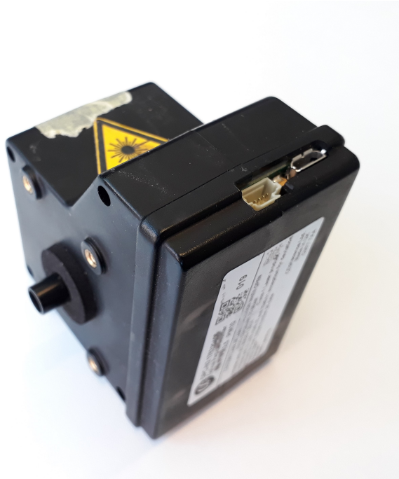
Figure 4: Alphasense OPC-N2 has four mounting holes spread around the inlet that make it easy to mount the sensor in enclosures. The sensor is also equipped with Molex PicoBlade connector for the serial peripheral interface (SPI) communication and a micro USB connector for access to the built-in SD card.
