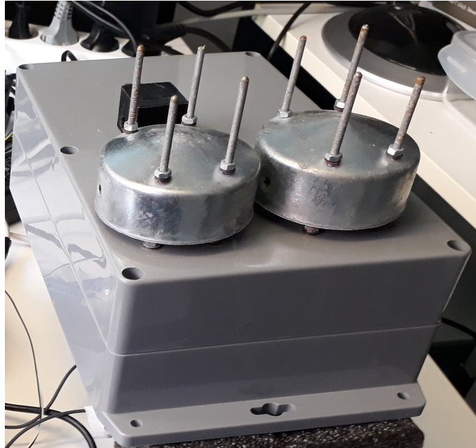
Figure 26: Measurement box used in the first field test. The pole caps protect the OPC-N2 inlets from wind and rain but leave a gap for the sample air. The small black box behind the pole caps is the protective case for temperature and humidity sensor.
