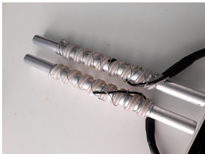
Figure 15: Heating cable wound around an aluminum pipe. The heating cable is held in place by steel wire. A small thermistor is placed on the heating cable and pipe with thermal paste.
