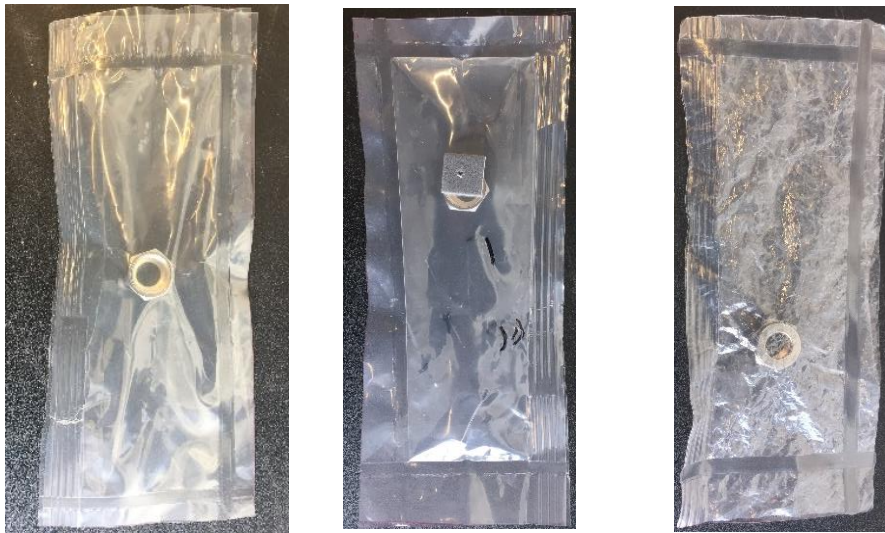
Figure 9: Micro-leak and burst test experimental setting (top) and PPCC1 samples tested (bottom, from left to right: unused, machine-folded and hand-folded)
