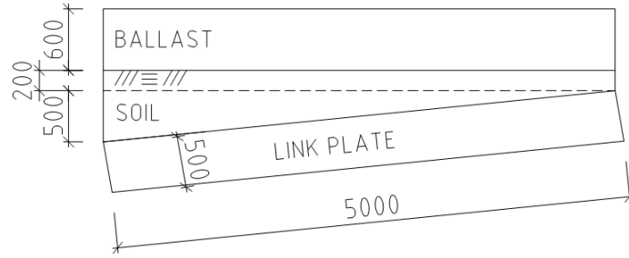
Figure B.3: Loads acting on the link plate. The width of the plate is 10.6 m.
