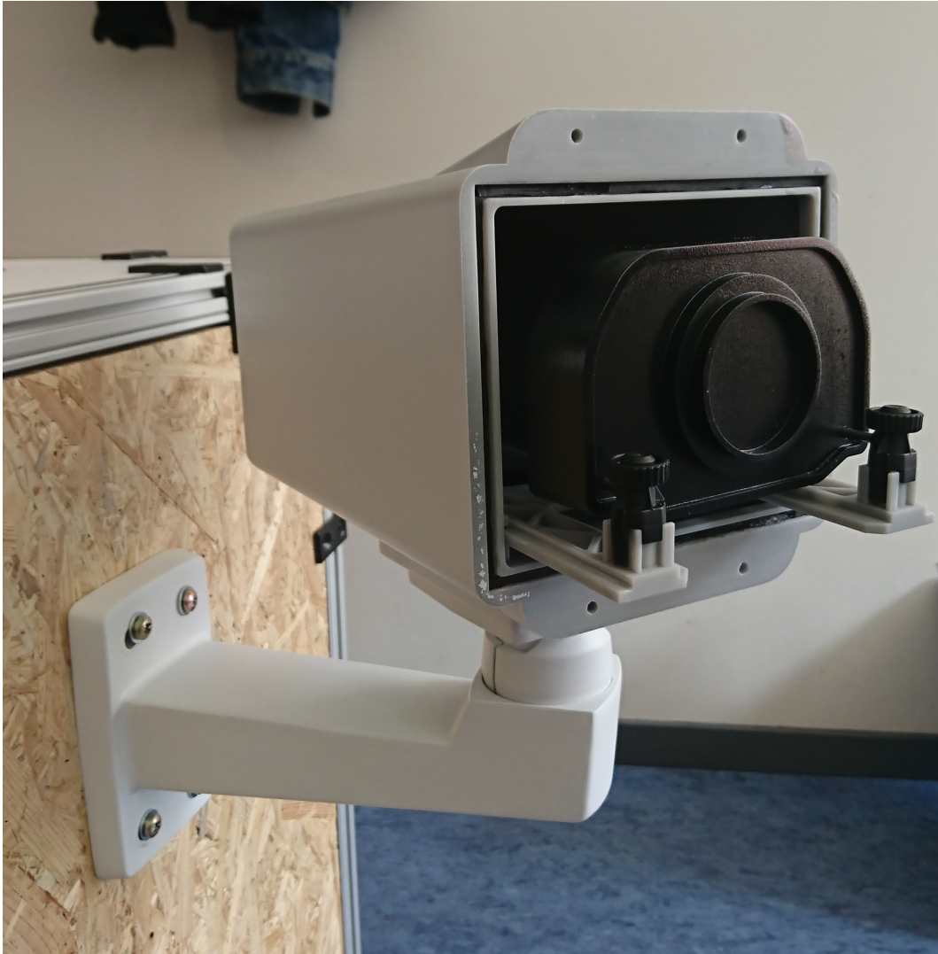
Figure 6.17: The final design of the assembled standardized housing with mounted camera sled.
