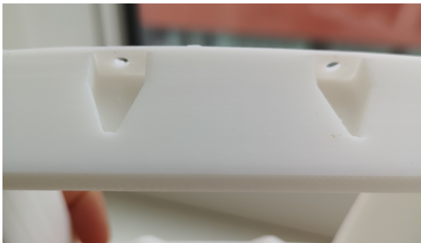
Figure 5.22: First 3D-printed prototype with tracks,screw holes B1.
