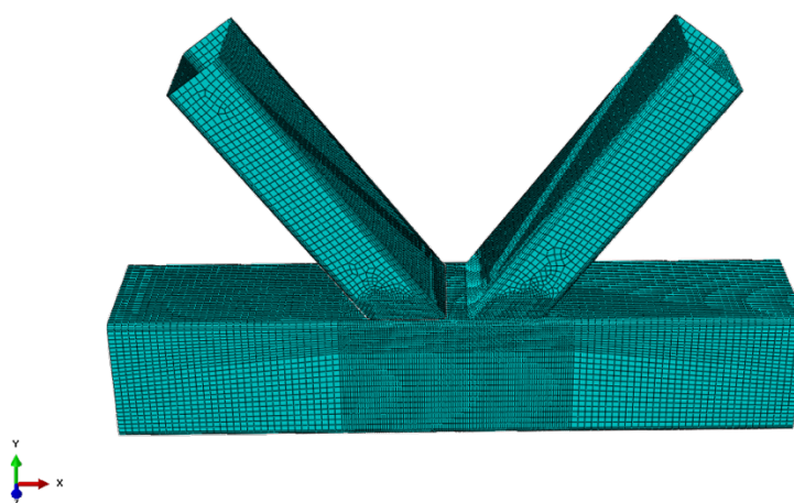
Figure 4.12 Locally refined mesh used for the elastic analyses.
