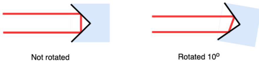
Figure 6: A schematic of a non-rotated and rotated corner gold mirror reflecting a laser beam.
