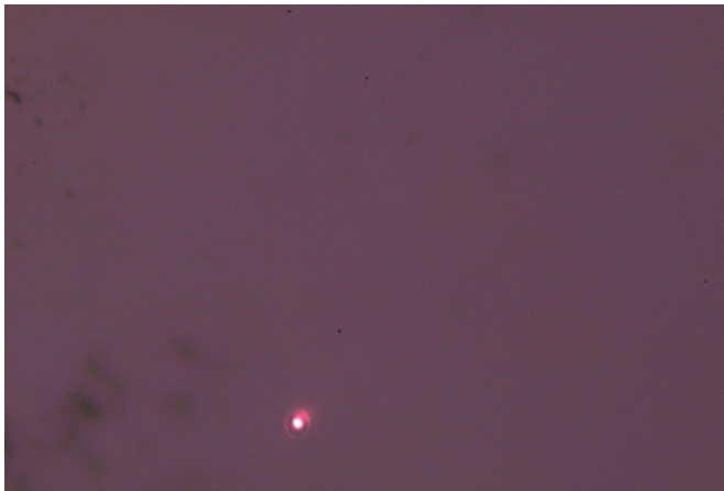
Figure 10: Picture from the microscope view when the laser spot was as visible as possible on the sample
