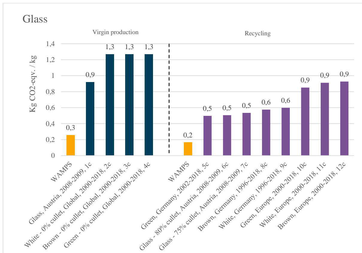
Figure 18. Presentation of the CO 2 -equivalents for glass production and recycling calculated by WAMPS and identified in literature/databases.
