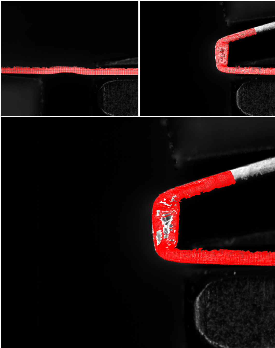
Figure 4.9: Mesh tracking material points. Top left: Initial mesh, 4 px spacing. Top right: Final mesh, 4 px spacing. Bottom: Final mesh with breaking, 2 px spacing.
