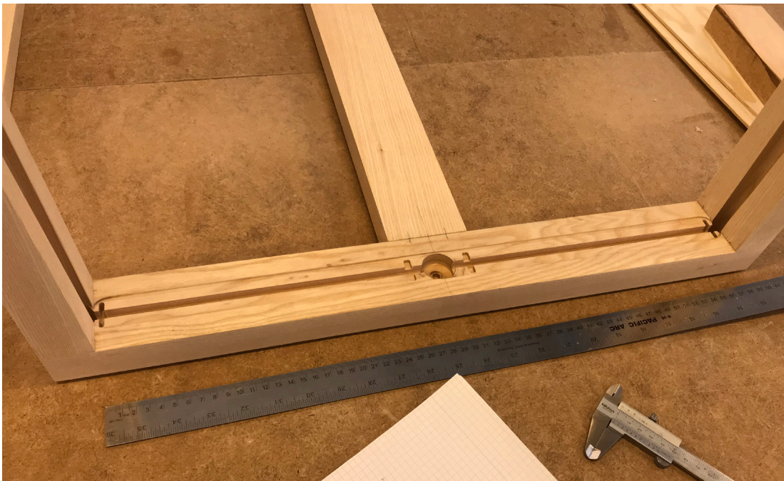
In the milled out groove a spring loaded hinge would allow the pins to lock and release.
