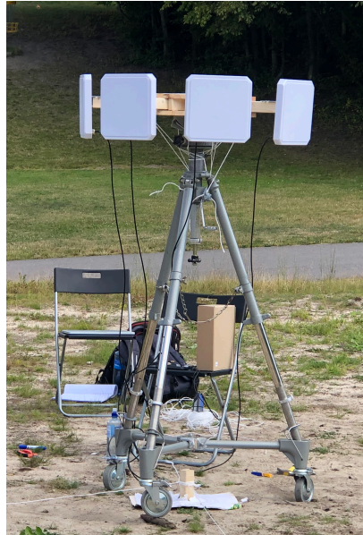
Figure 5.2: Antenna Holder and Four Antenna Setup.
