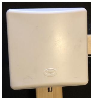
Figure 4.7: Physical appearance of Panorama W24-58-CP-9 directional antenna.
