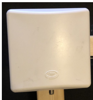
Figure 4.7: Physical appearance of Panorama W24-58-CP-9 directional antenna.
