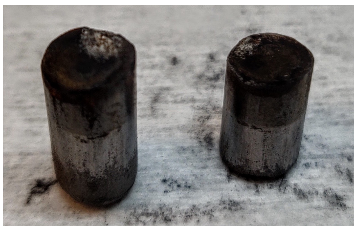
Figure 4.3: Photograph of two stainless steel electrodes pressed at 100 bars after being used in the SDG with the end exposed to the spark discharge facing up. Note the light silver colour on the top of the electrode indicating where the spark ablates material from the electrode.
