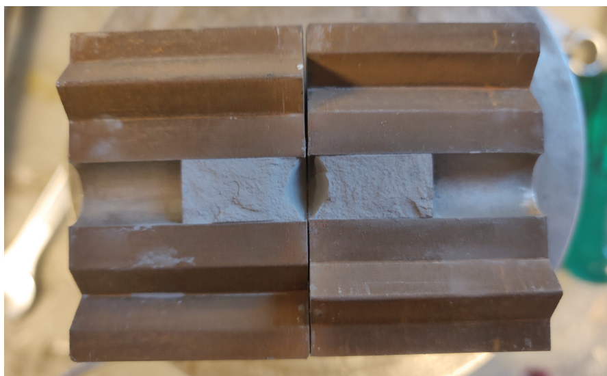
Figure 4.4: Two halves of a stainless steel electrode pressed at 100 bars stuck in the chamber of the second block tool.
