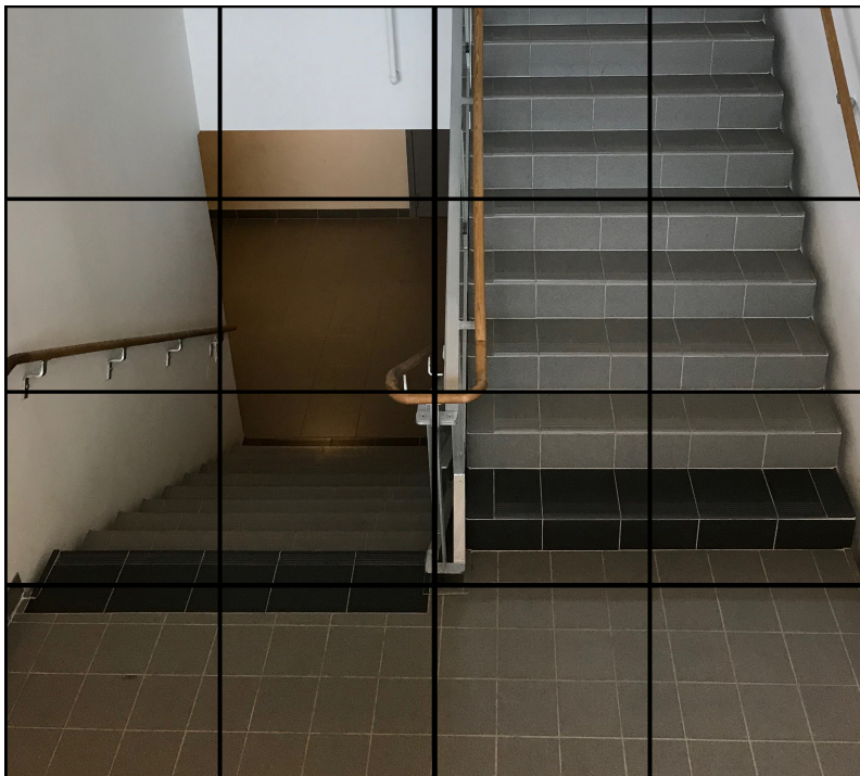
Figure 2.7: A block based representation of entry/exit zones in the FOV showing a stairwell.
