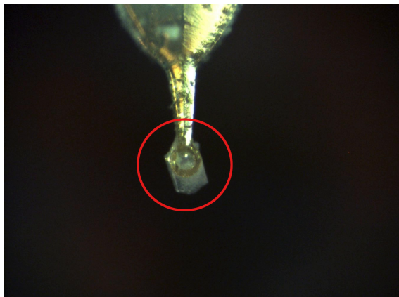
Figure 2.2: A loop holding a crystal, seen from the perspective of the beam source.
