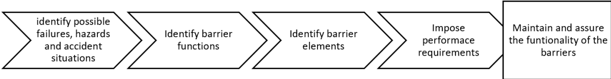
Figure B 8: Key steps in barrier management, the picture is an altered version of the original from “Principles for barrier management in the petroleum industry; Barrier Memorandum 2017” (Petroleum Safety Authority Norway, 2017a, p. 11).
