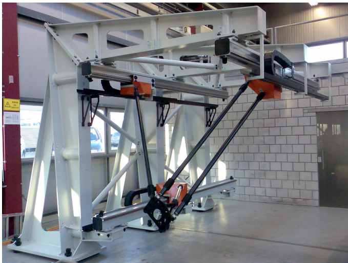
Figure 1.1 Gantry-Tau prototype, where the three orange carts were controlled along their rails to move a tool along a desired trajectory [SMErobot, 2009].
