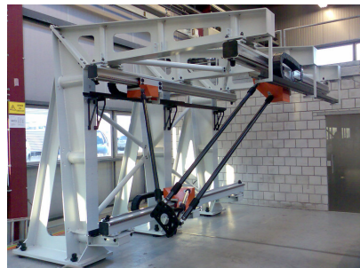
The Gantry-Tau robot where the robot joints can be seen in orange.
