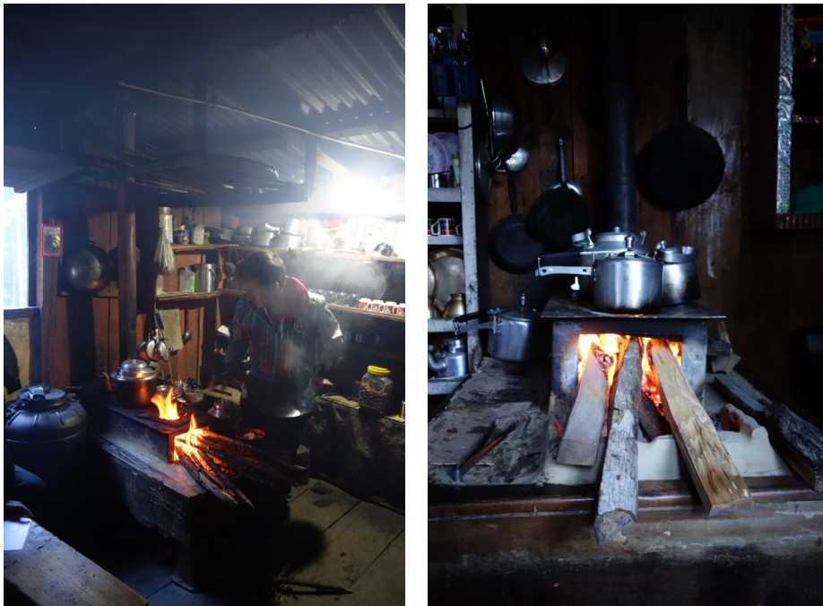
(a) Combustion of firewood taking place outside the combustion chamber. (b) Firewood logs gradually metered into the fire.
