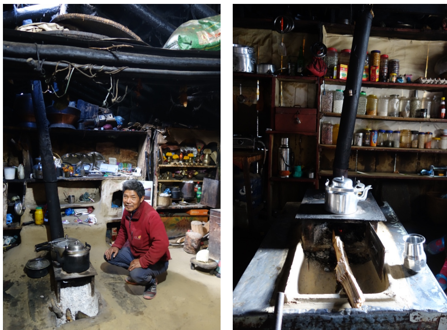
(a) Locally manufactured metal stove. (b) Subsidized metal stove with fire gate.
